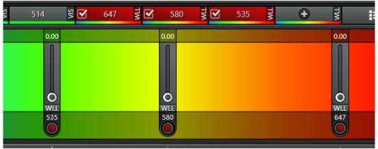
b. WLL-specific: To add more WLL lines click "+". Double-click on the wavelength to change it or slide the laser bar to the correct wavelength (B). Set the intensity to 1% to start and make sure the circle below the wavelength (D) is red (shutter ON).
