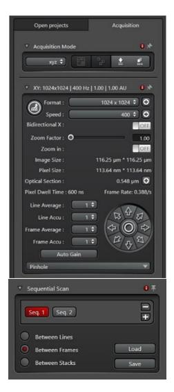
When imaging on sequential mode: All lasers should be <u>always on</u> (red button) but lowered to 0% during the sequences that are not needed.
