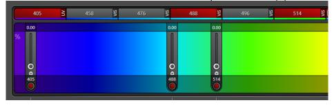
i. For the WLL, click "+" to add up to eight additional laser lines (practical advice: do not exceed 2-3 lines). WLL lines must be further activated by adding a checkmark next to the laser line. Lastly, activate the red indicator under the laser line and double-click on the number to set the precise excitation wavelength.
